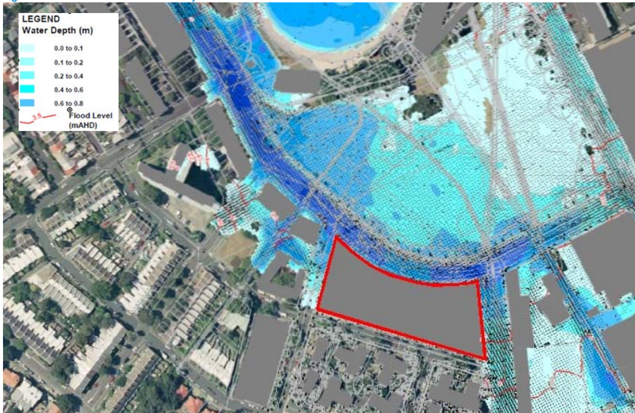
Figure 2.1 – Peak Flood Levels 100yr ARI event
